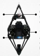
The carbon cage makes the Spy II very robust and resilient to impacts. Its conical shape allows it to easily navigate through obstacles.
